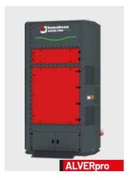
ALVERpro Series air tower units are specially designed air towers which apply layered ventilation system by sucking the dirty air from the top and releasing the clean air with low velocity from the bottom. ALVERpro smart cleaning technology ensures superb filter cleaning efficiency and extend the filter life time. VFD driven fans allows users to regulate the air speed upon their need.
